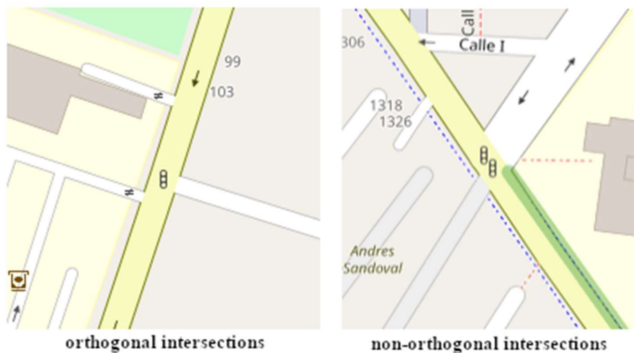
Fig. 2. The intersection is orthogonal when the street angle is between 85 and 95 degrees, and otherwise, the intersection is non-orthogonal. The left side of the figure shows orthogonal intersections, while the right side contains non-orthogonal intersections [9].
